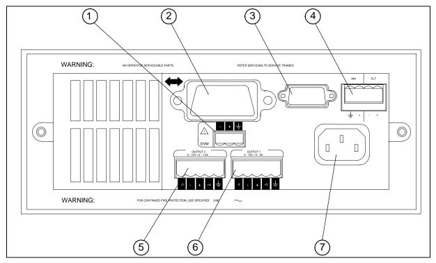
**5** Output 2 connector (Agilent 66309B/D only). Connector plug is removable.
